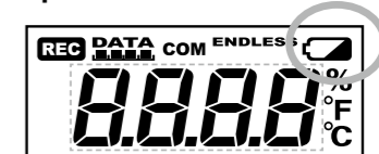
Battery Warning Mark
