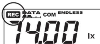
Press the REC/STOP button until the [REC] mark appears in the display.
