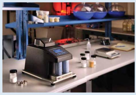
instrument capable of both dynamic and static methods, and the breadth of moisture sorption data that can be generated using the VSA will significantly contribute to improved understanding of water-solid interactions."
