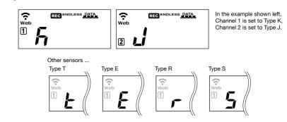
The factory default setting is "K" for both 1 2. Depending on the thermocouple type you're going to use, make settings or changes using "T&D WebStorage Service" or the software "TR-7wf/nw for Windows".
